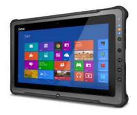
The Getac F110 is powered by an Intel Core i5-5200U (2.2GHz) or i7-5500U (2.6GHz) processor, 4GB RAM, and a 128GB solid state drive. The Getac F110 has built-in 802.11ac WiFi, Bluetooth 4.0, and optional 4G LTE Mobile broadband to keep workers connected. The optional webcam and 8MP autofocus camera can capture images or video on the go.
